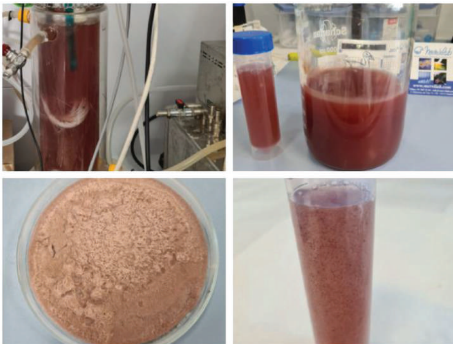
Figure III.7 Photos showing MPBR (top left), biomass collected at S2 (top right), lyophilized biomass (bottom left), and granulated biomass collected at P3 (bottom right).
