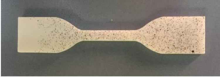
Figure 4-4. Tensile specimen painted with a random dot pattern.
