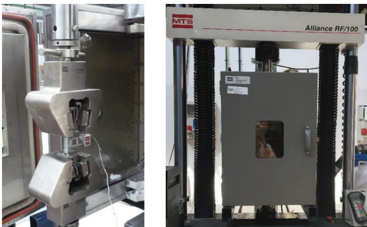
Figure 4-3. MTS Alliance RF/100 with environmental chamber MTS 651.06E-03 and load train installed for tensile tests at -50 °C and 50 °C.
