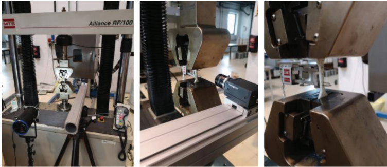
Figure 4-5. MTS Alliance RF/100 equipped for tensile tests at room temperature, with contact extensometer MTS 634.12F-54 and VIC 2D videoextensometer.
