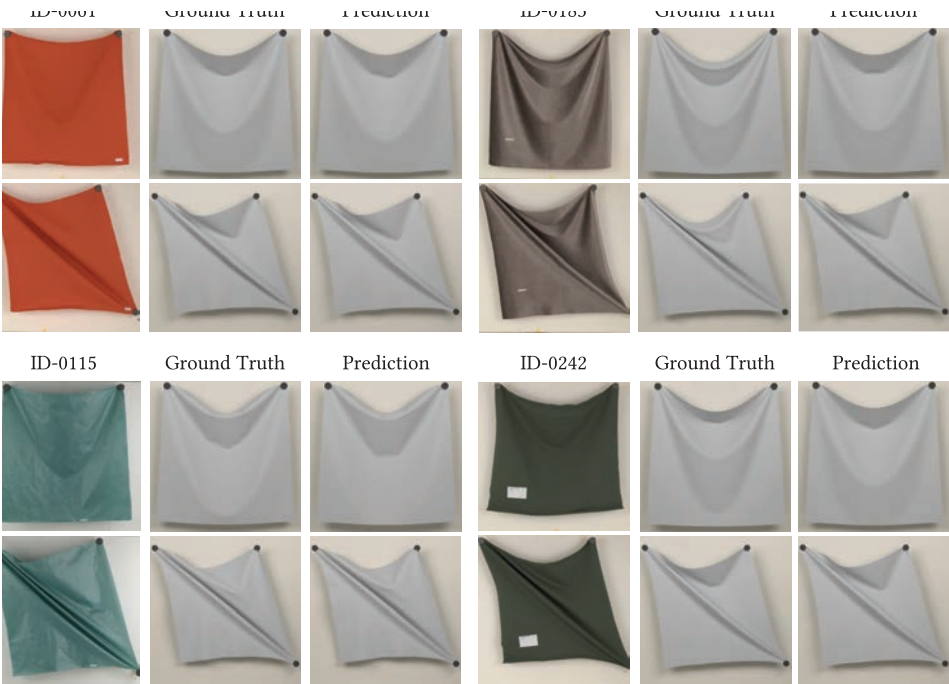
Figure 6.10: A comparison between the simulations obtained through the ground truth parameters, and those obtained using the predictions of our model, from a representative set of fabrics of our test set. As shown, the estimations of the model yield similar drapes to those of their ground truth counterparts, which we also evaluate quantitatively.
