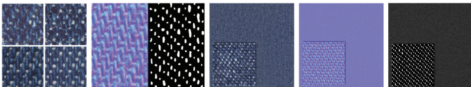
Figure 2.1: Illustration of the capabilities of our attribute transfer framework. On the left, we show a subset of our photometric dataset , comprised of several images of a material captured with different illumination conditions. On their right, two visual attributes: surface normals and segmentation maps. Using a larger image of the same or similar materials as guidance , our method can propagate the visual attributes, achieving high resolution, robust and controllable transfers at small computational cost.
